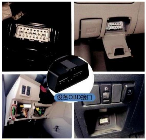
**Note:** The OBD interface positions of different models are different. The following figure shows the possible locations of the OBD interface. Some vehicle OBD ports are hidden behind the plastic baffle:
